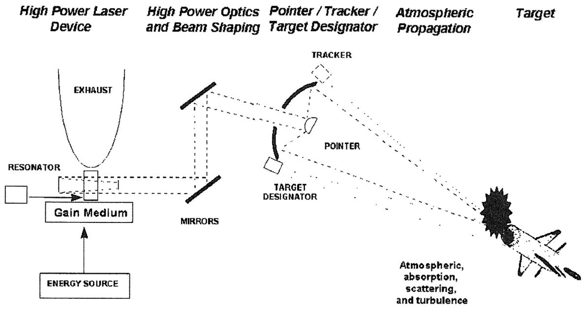
Figure 2. Elements of an HEL Weapon System
