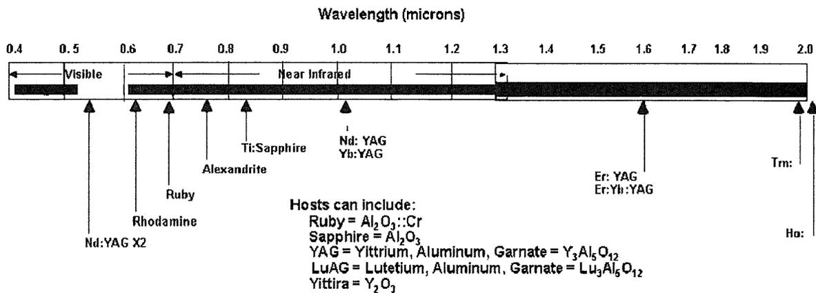
Figure 5. Common Solid-State Lasers and Their Wavelengths
