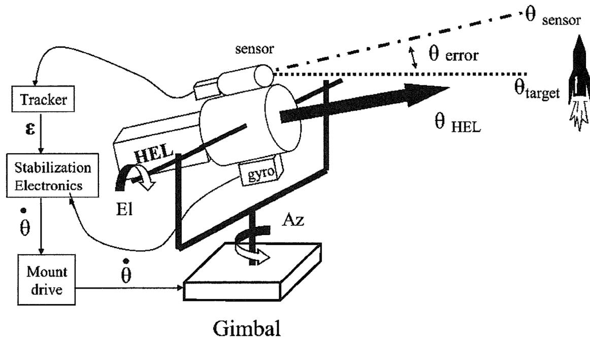
Figure 10. HEL Weapon Basic Tracking and Pointing Controls
